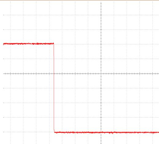
The soft start of shutdown by both power supply and the switch. When the current is 1A, the voltage is 6V.
