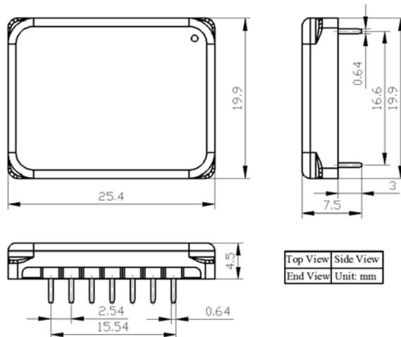
Figure 13. Dimensions of the DIP Package Driver
