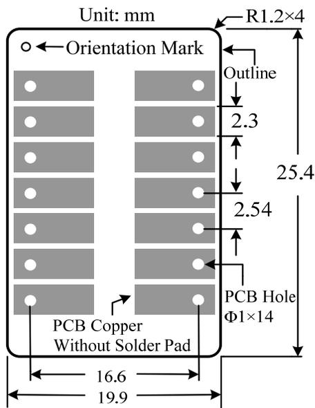
Figure 15. Top View of the Top Side PCB Foot-print
