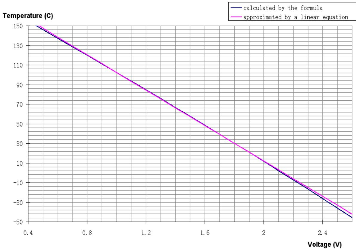
Figure 5. Controller Internal Temperature vs. TMPO Voltage
