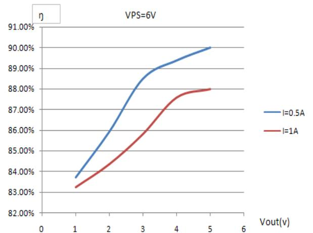
Figure 11. Efficiency of Laser Driver
