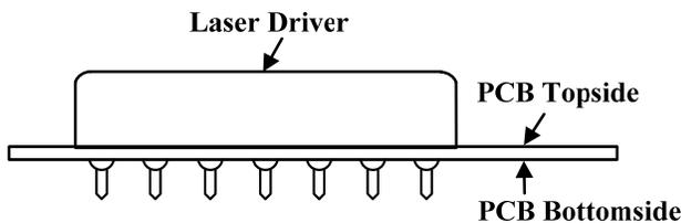
Figure 16. End View of the PCB Foot-print
