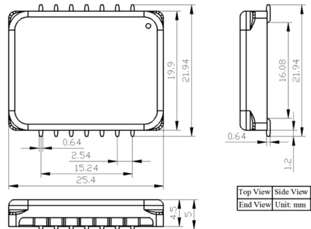
Figure 14. Dimensions of the SMT Package Driver
