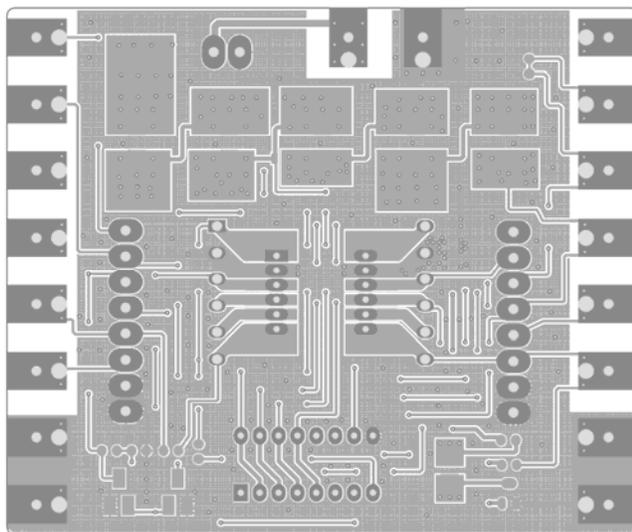
Figure 4. Top Layers without Top Screen Layer
